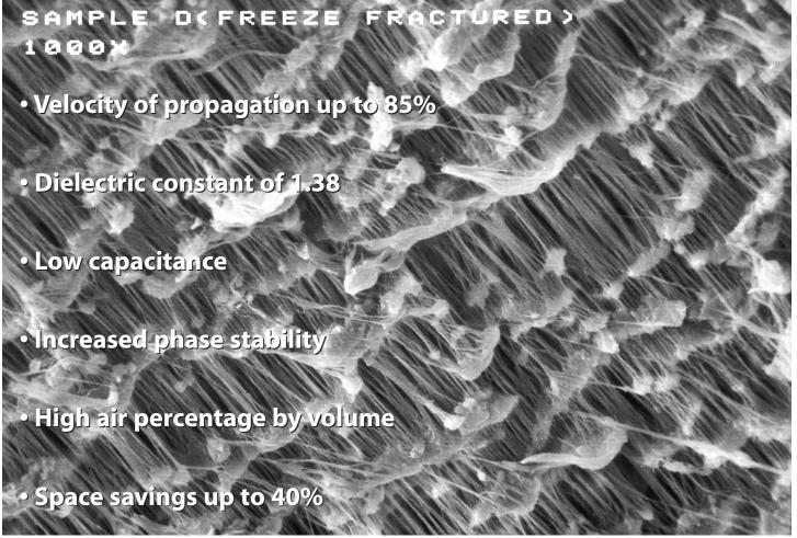
Thermax **LTE** is a patented extruded expanded low-density PTFE dielectric offering multiple advantages, not only over solid PTFE, but other air-spaced constructions as well.
